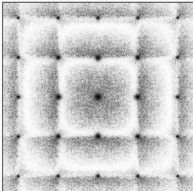
**Fig. 3.** An example pattern which demonstrates the size effect in a cubic two-component alloy: The smaller atom has the higher scattering power. The diffraction pattern is calculated with DISCUS [29].
